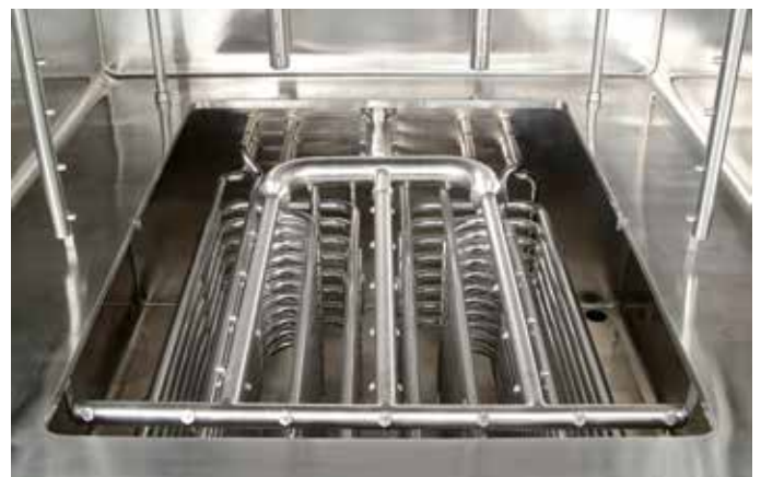
Ice condenser chamber with CIP-/SIP-piping
