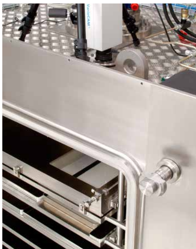
Modification of a freeze dryer for bulk API in order to support use of an IR camera for process monitoring combined with adjustable shelf spacing
