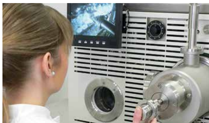
Lab technician removing samples during the ongoing FD process
