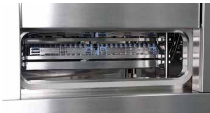
Frames which can be automatically cleaned and sterilized by CIP/SIP in the freeze dryer
