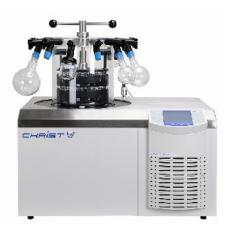
Two heatable shelves with stoppering device, additional connections for twelve round-bottom flasks, wide-neck bottles or ampoule distributors Condenser capacity: 16 kg Condenser temperature: -85° C
