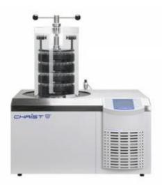
Four heatable shelves with stoppering device Condenser capacity: 16 kg Condenser temperature: -85° C
