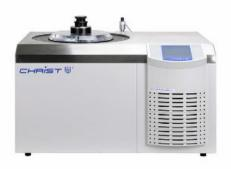
Freezing and drying inside the ice condenser (single-chamber method) on five heatable shelves, optionally with a fan Condenser capacity: 16 kg Condenser temperature: -85° C
