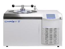
Freezing and drying inside the ice condenser (single-chamber method) on two heatable shelves with stoppering device, optionally with a fan Condenser capacity: 16 kg Condenser temperature: -55° C
