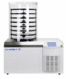
Eight heatable shelves; optional lifting device for drying chamber available Condenser capacity: 16 kg Condenser temperature: -55° C
