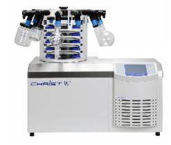
Five heatable shelves, additional connections for twelve roundbottom flasks, wide-neck bottles or ampoule distributors
