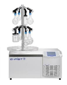
Drying manifold for eight round-bottom flasks, wide-neck bottles or ampoule distributors; specifically suitable for solvent drying
