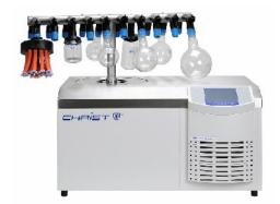
Drying manifold for up to twenty round-bottom flasks, wide-neck bottles or ampoule distributors; specifically suitable for solvent drying
