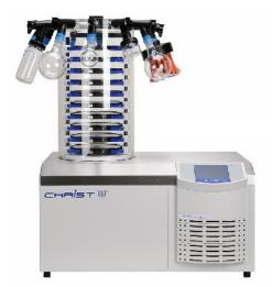
Ten heatable shelves, additional connections for twelve roundbottom flasks, wide-neck bottles or ampoule distributors
