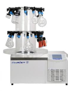
Two drying chambers with a total of 24 connections for roundbottom flasks, wide-neck bottles or ampoule distributors Condenser capacity: 8 kg Condenser temperature: -55° C
