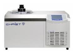
Freezing and drying inside the ice condenser (single-chamber method) on a heated shelf, optionally with a fan Condenser capacity: 8 kg Condenser temperature: -55° C
