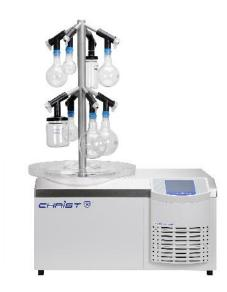
Drying manifold for eight round-bottom flasks, wide-neck bottles or ampoule distributors; specifically suitable for solvent drying Condenser capacity: 8 kg Condenser temperature: -55° C
