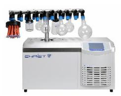
Drying manifold for up to twenty round-bottom flasks, wide-neck bottles or ampoule distributors; specifically suitable for solvent drying Condenser capacity: 8 kg Condenser temperature: -55° C
