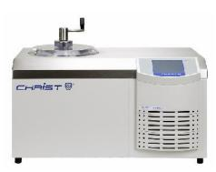
Freezing and drying inside the ice condenser (single-chamber method) on a heated shelf with stoppering device, optionally with a fan Condenser capacity: 8 kg
