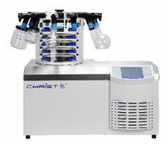
Five heatable shelves, additional connections for twelve roundbottom flasks, wide-neck bottles or ampoule distributors Condenser capacity: 8 kg Condenser temperature: -55° C
