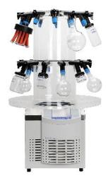
Two drying chambers with a total of 24 connections for round-bottom flasks, wide-neck bottles or ampoule distributors
