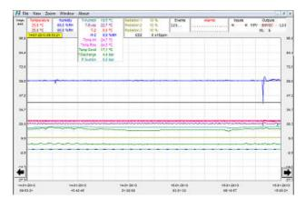
**FitoLogView:** It is a working tool to process the data recorded by the FitoLog program. One can view, print and export the log contents to other file types, and analyse the data in other data management software (Excel, Star Office, Access or others).
