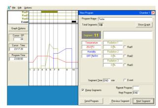
**FitoProgram:** This application simplifies the creation of programs and its integration on the chamber ClimaPlus controller. Up to 32 programs, each with 24 segments, can be designed and linked to create detailed environmental profiles and simulations.
