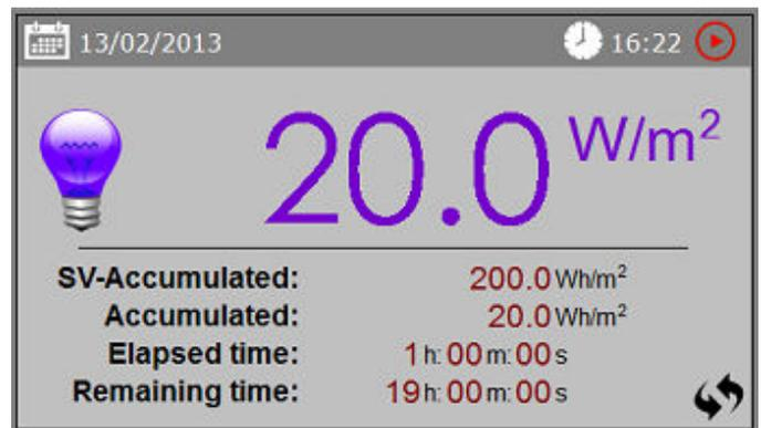
ClimaPlus controller specific for the Photostability chambers with automatic integration of VIS and UV sensors and radiometer according to traceability standards. Enables automatic running (with auto-stop) of test programs and FDA 21 CFR compliant data logging
