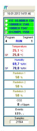
**FitoLog:** Displays and records in real time all data and details related to the set-points, running variables and equipment behaviour. It also retrieves information about the active components of the chamber, running processes, errors, alarms and allows the configuration of periodic or alarm triggered remote notifications (by email or SMS, depending on existing connections and accessories).
