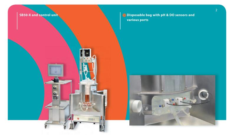
The SB50-X is an orbital shaken bioreactor for the cultivation of human, mammalian and plant cells in a disposable bag. A working volume from 15 litres up to 50 litres for the SB50-X ensures easy scale-up from microtiter plates to shaking flasks and all the way up to 200 litres. The SB50-X can be used in research, process development or production.
