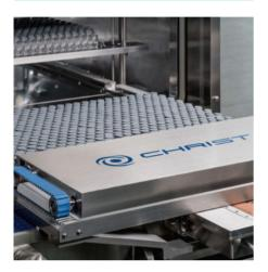
The LyoShuttle robot pushes the vial package on the shelf.
