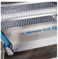
The LyoShuttle robot pushes the vial package out of the freeze dryer.
